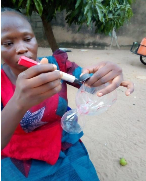
Plate 17: Making designs along edge of plastic bottle using marker before trimming.
